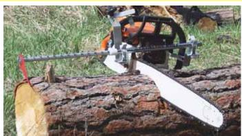
The Chainsaws Rule allows you to measure the wood as you cut it. Telescoping rod has 1-in. markings on it and a red aluminum flag at one end.
