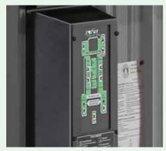
The FireStar II controller controls the outdoor wood furnace and can store data and communicate with other devices.
