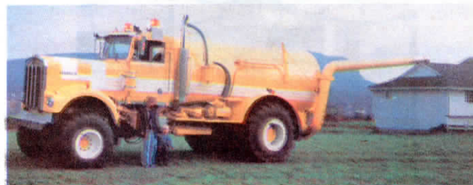
Van Jaarsveld also built 2,500-gal. manure tanker mounted on Kenworth semi body.
