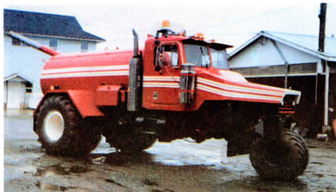
To build 1,500-gal. flotation sprayer, Van Jaarsveld first stripped 1975 GMC 5-ton truck down to frame. He fashioned the narrow, front sloping hood out of sheet metal.
