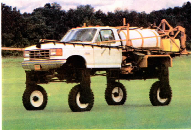
"Stilted" sprayer has 39 in. of crop clearance. Can be switched back to normal operation in 3 hours.
