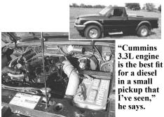
Jacob Kraybill repowered this Ford Ranger with a Cummins 3.3L industrial engine, building an adapter ring to connect the diesel flywheel with the flywheel from the Ranger's original gas engine.
