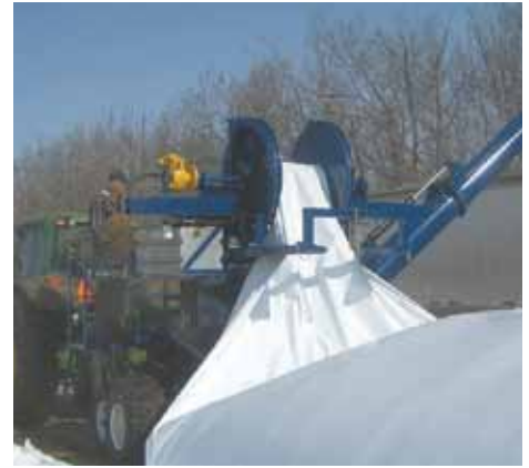
Neeralta Mfg.’s new grain extractor can unload a 9 to 12-ft. dia. grain bag at up to 150 bu. per min., then roll the empty plastic bag up into a neat 30-in. wide roll.
