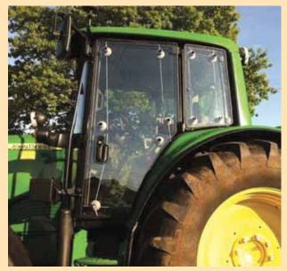
**Tractor Guard** window protectors are designed to protect your tractor's windows and mirrors from flying rocks and trash.
