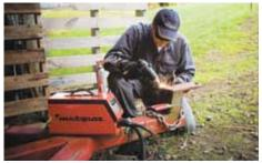
Not much bigger than an old-time radio, all the Multiplaz 3500 welder needs is 110 or 220-volt current, water and alcohol.
