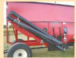
New-style 18-ft. auger can reach out 28 ft. in front and 55 ft. from side to side to fill planters and grain drills. Auger folds down within the length and height of most gravity boxes.
