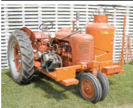
SC Case tractor belt-drives an air compressor on one side of tractor, which feeds air into a big 200-gal. tank on other side.
