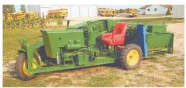
The operator rides in comfort on a cushioned chair while steering a single front wheel. Foot and hydraulic controls are within easy reach.
