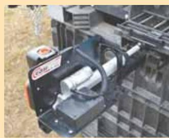
Remote-controlled seed box opener uses an electric actuator to open and close the slide gate on bulk boxes.
