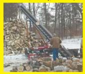
We cut a lot of firewood to heat with but we got tired of stacking the split wood. So we powered a corn elevator with a Briggs & Stratton engine through a gear reduction unit. It works great and sure saves time and back pain. (Leon Dahle, 407 N.W. 4<sup>th</sup> St., Morristown, Minn. 55052 ph 507 685-2245; dsf@ bevcomm.net)
