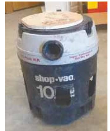
Converted 10-gal. Shop-Vac has several feeding ports cut into the side.
