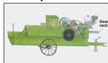
All mechanical wood shavings baler works faster than hydraulic balers. It uses a rack and pinion to run the plunger back and forth.
