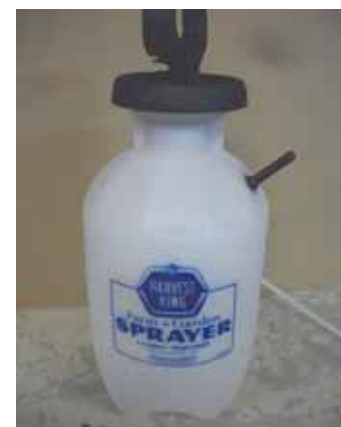
Add-on automotive valve stem lets Dwayne Slate use an ordinary air compressor to pressurize his hand sprayer tank.
