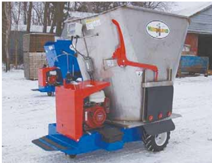
Vertablend self-propelled mixer cart is small enough to deliver mixed rations to livestock in older tiestall barns.
