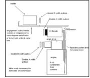
Erling Brakefield turned an old Massey Harris pull-type combine into this mobile power source that's fitted with a compressor, welder and generator.
