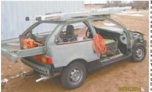
Drawdy removed car's doors, seats and rear hatchback, then built a plywood platform on the passenger side and on back. Wooden rack on top is used to haul a ladder or other cargo.
