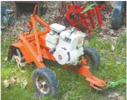
To convert rear tine tiller to a tow-behind model, Russ Wing replaced the tiller's self-propelled wheels and added an offset hitch.
