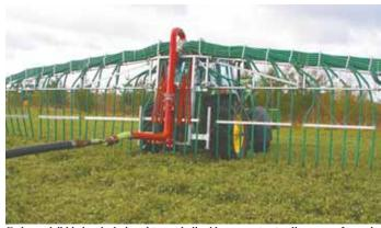
Cadman dribble bar is designed to apply liquid manure to standing crops. It can be used on any crop that can be sidedressed, including corn at early stages.
