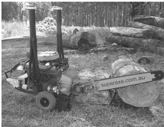
Australian David Burder took the backbreaking work out of this big saw by mounting it on wheels. It's powered by a Holden 4.2-liter, V-8 car engine.
