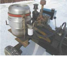
A beer keg attached to Robert Ingerson's wood splitter makes a practical . hydraulic fluid reservoir. "It's great because it's stainless steel and has an internal baffle. It holds a lot of oil. keeping it cool," he says.
