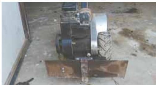
Steel plate attaches on front of rear-end rototiller. Brandt tills a long strip with the tiller in the ground and the plate up in the air. Then he puts it in reverse, lifts the tiller and goes backward to smooth out the soil. Pointed blade on front digs a seed furrow.
