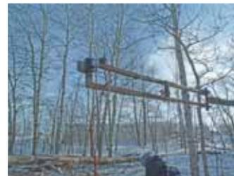
Crane consists of an 8-ft. upright with a 2-part boom (left). A section with a 12-volt winch mounts at end of boom.
