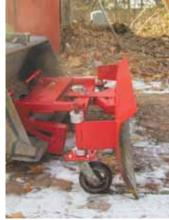
"It attaches to the loader bucket like a giant C-clamp and mounts on 8-in. caster wheels so it can float," says Jake Clark about his home-built, bucket-mounted blade.
