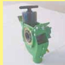
Nozzle shield installed over a seed cup.
