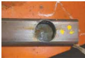
Plasma Pro templates can be clamped or spot-welded in place, ensuring the hole you cut is exactly where you want it.
