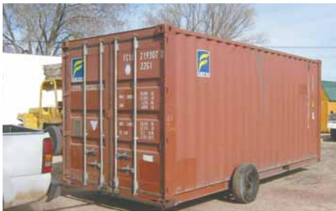
Ken Dobson used scrap metal and axles from an old motorhome to make a dolly system for moving metal shipping containers.
