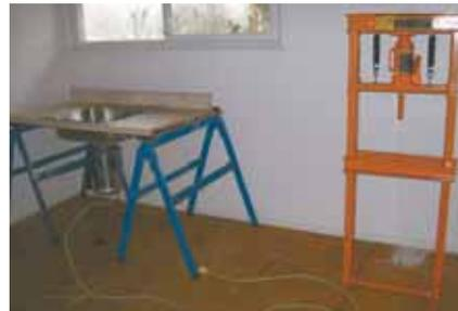
**Garbage disposal, left, is used to grind up olives and pits into a mash and hydraulic press, right, extracts the oil.**
