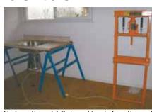
Garbage disposal, left, is used to grind up olives and pits into a mash and hydraulic press, right, extracts the oil.
