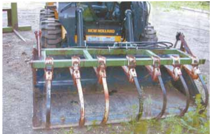
Harlen Grovom used part of the frame and some shanks from an old field cultivator to build this grapple fork. He bolted it to the bucket on his New Holland skid loader.
