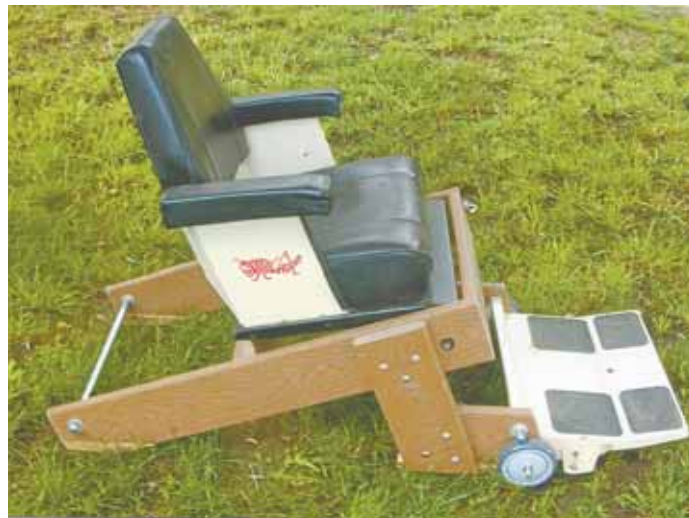
Lawn chair is fitted with the seat off a Grasshopper riding mower. With wheels on front and a grab bar on back, it can be easily moved to wherever it's needed.
