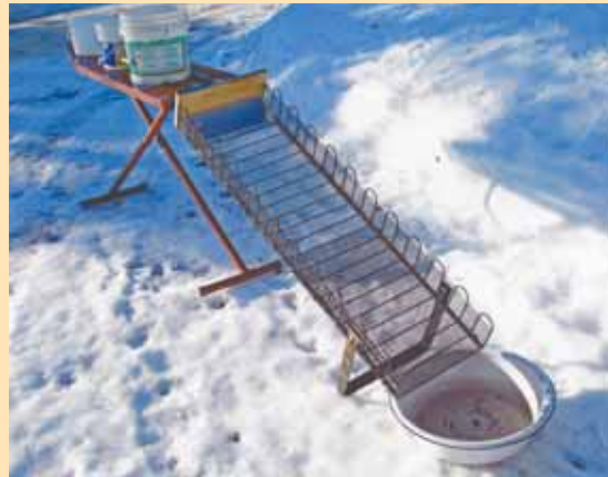
Berry cleaner uses the heat transfer screen from the back of an old refrigerator. Leaves and stems fall through to the ground and the clean berries roll down into the bowl.
