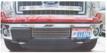
Dan Thornburg used 5/16-in. thick stainless steel to build this grille on front of his new Ford F-150 EcoBoost pickup. It protects the vehicle's turbo intake.
