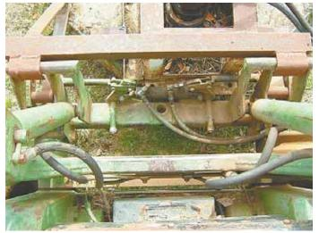
Mower was originally mounted under the belly of a Cub Farmall. Kimball replaced the pto drive with a hydraulic drive and hinged the mower deck to the frame.
