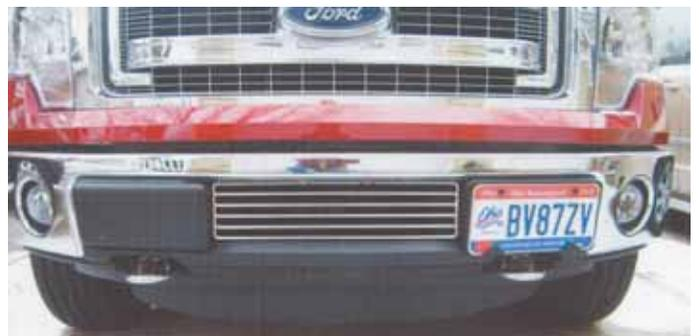
Dan Thornburg used 5/16-in. thick stainless steel to build this grille on front of his new Ford F-150 EcoBoost pickup. It protects the vehicle’s turbo intake.
