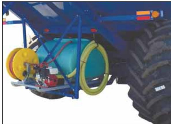
**Skid plate-mounted Enduraplas fire fighting kit is ideal for mounting on grain carts. Photo shows kit rear-mounted on a Brandt grain cart.**
