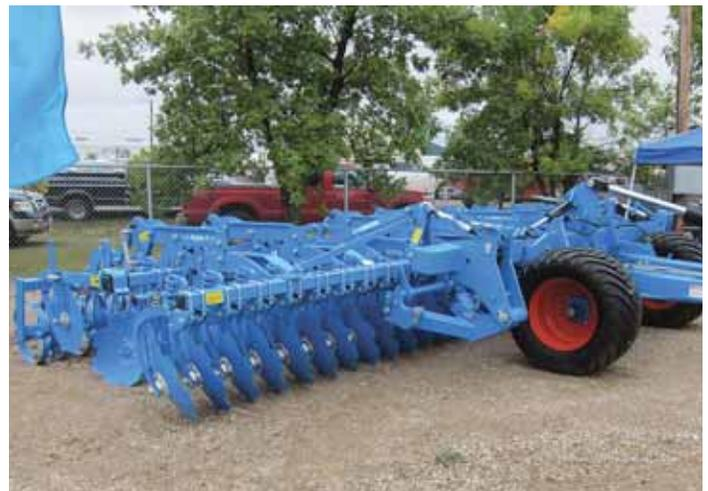
Discs on the Lemkin Rubin 9 disc harrow have a dual angle built into them, a combination that guarantees intensive mixing across the full working width.
