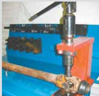
vice can be a challenge because it's hard to hold them in place while turning the handle. After 30 years of working with pto's and drivelines, we've developed a 'C' frame press that uses a special hydraulic jack and custom tooling to press bearing caps out of yokes; press bearing caps out of yokes to save the cross and bearing set; install a new cross and bearing kit; and hold pto halves so the safety shield can be removed.
