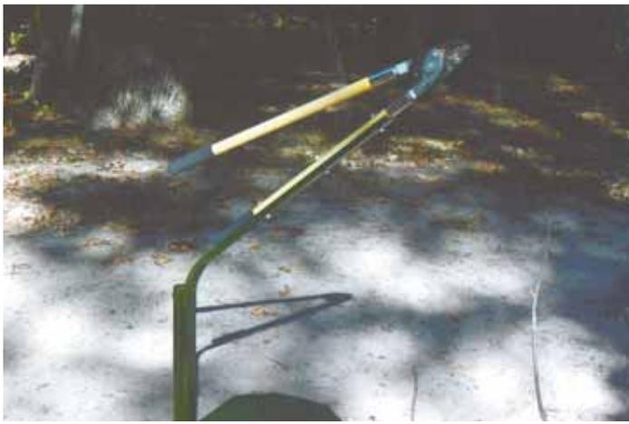
“One-handed branch cutter” lets Jacobson hold a tree branch in one hand and chop it with the other.
