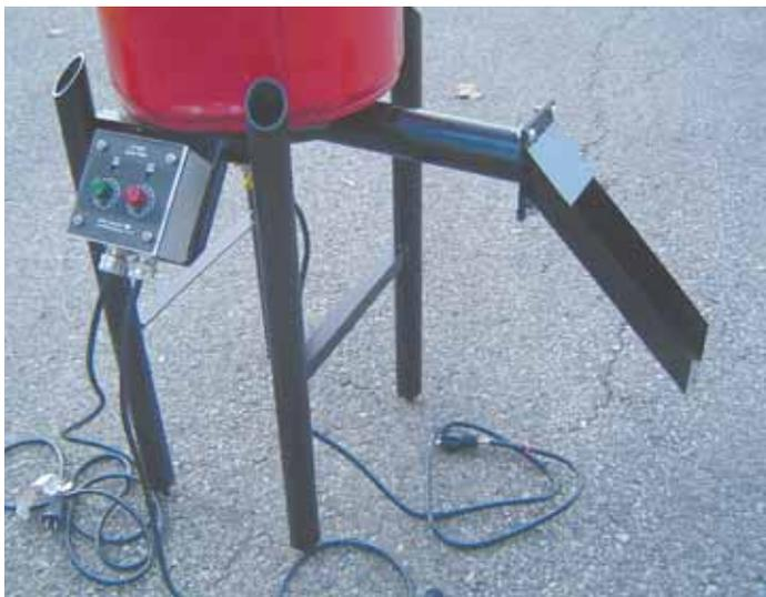
Carl Dobrovolny sells parts to make your own pellet stove or to upgrade an existing stove to totally automatic operation. Parts include this Cycle Timer/Auger Control.
