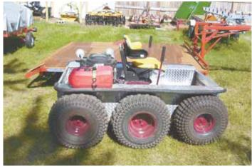
Jim Tesmer's home-built, amphibious 6-wheeler uses the drive unit off a zero-turn Ariens mower.
