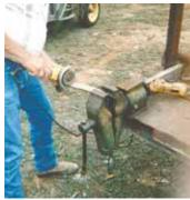
He cuts grooves 1/4 in. deep every 3/4 in. on the cutting edge of the blade.
