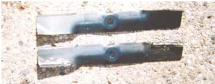
Darrell Longman boosted the suction power of the blades on his Deere lawn tractor, by welding a 1/4-in. square rod to the back side of each blade’s cutting edge.
