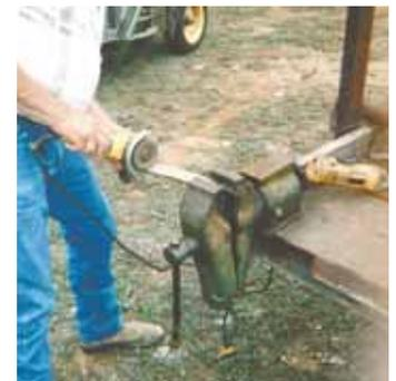
He cuts grooves 1/4 in. deep every 3/4 in. on the cutting edge of the blade.
