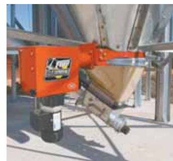
To keep feed moving, Flow Hammer delivers 500 lbs. of force every second to a metal band attached around bin collar.
