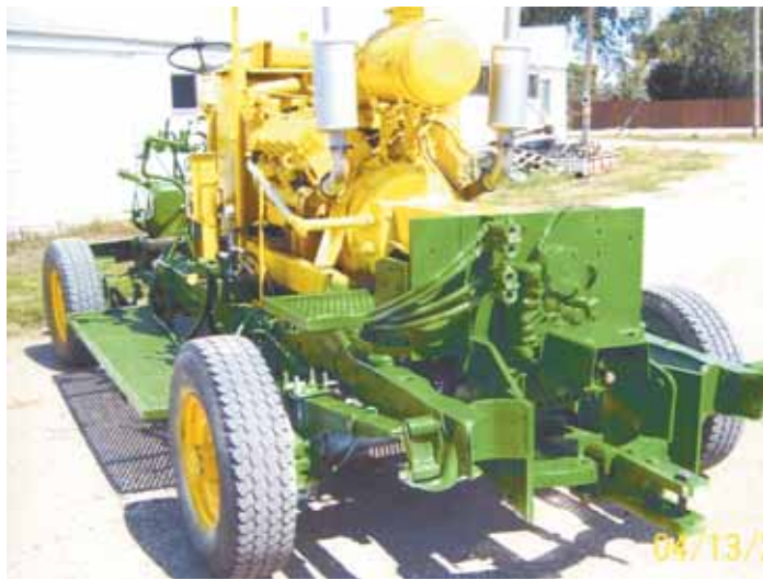
Pto shaft and drawbar on front, allows Perrion to push an auger up to the bin, raise or lower it, and operate it. Hydraulic outlets can be used to operate a belt conveyor.
