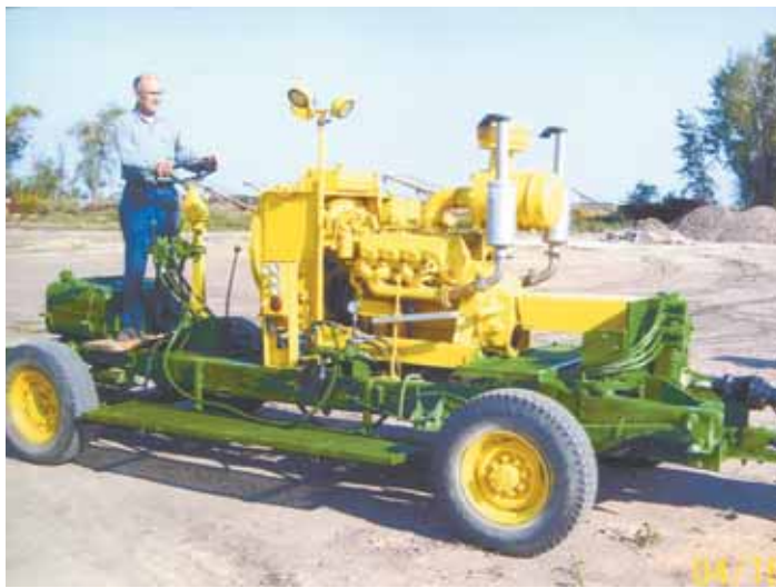
Don Perrion built this self-propelled “pto power plant” that eliminates the need for a tractor. The 2-WD rig is powered by a 170 hp Cat diesel engine.
