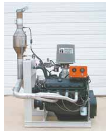
Dual fuel system mixes diesel fuel and natural gas as it enters the injection system of a diesel engine.
