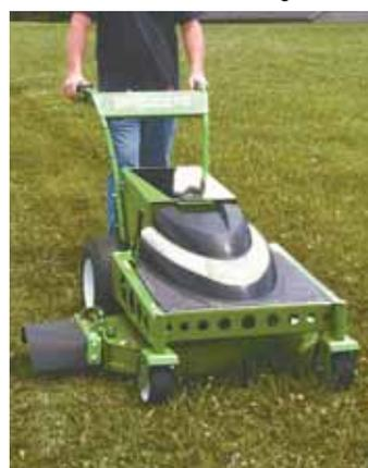
Walk-behind, 33-in. wide electric mower runs on a lithium energy module power pack.
