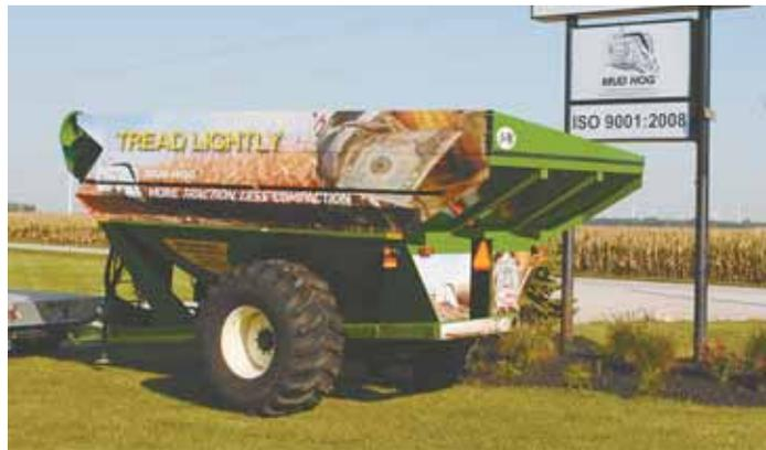
Grain carts equipped with Mud Hog 2-speed hydraulic-driven axles reduce both fuel use and compaction, says an Indiana company that offers the axle drive on J&M grain carts.
