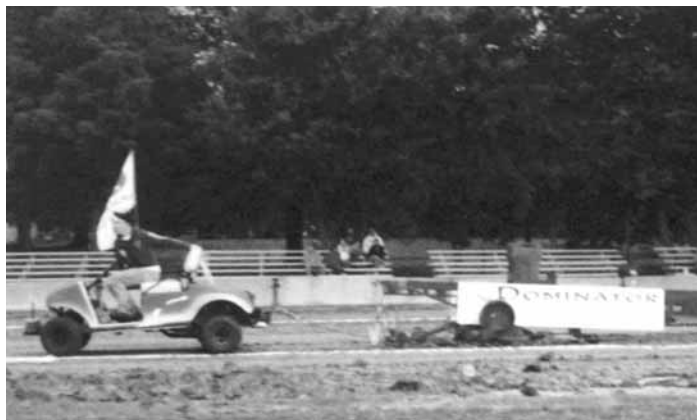
Home-built golf cart sled is a scaled-down version of a full-size tractor pulling sled. Golf cart shown was repowered with an 18 hp Briggs Vanguard engine.
