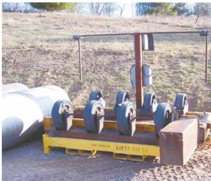
Machine cradles tank on 8 rubber wheels – 4 idlers and 4 drivers – and rolls tank while it's being cut with a plasma cutter that mounts on a metal arm.
