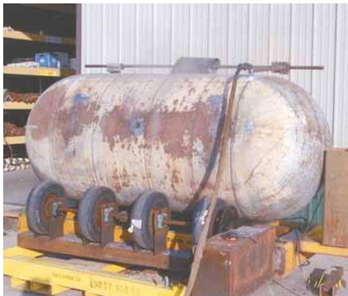
Home-built machine is designed to cut old 500-gal. LP tanks into fire rings, burn barrels, and more.
