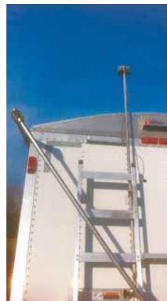
Each video camera is attached to a telescoping metal conduit that extends 2 to 3 ft. above the top of Jim Case's semi truck grain trailer.
