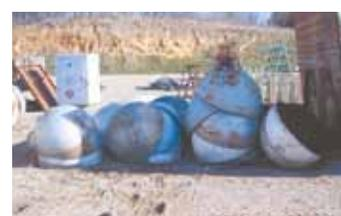
Schley cuts fire rings from 12 to 18 in. high (left). On other tanks he cuts off one end to make boilers, or both ends to make culverts.
