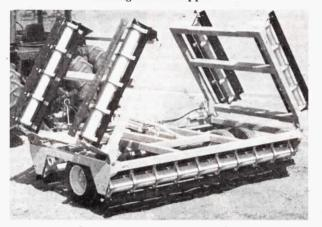
Two gangs of ground-driven rolling chopper blades on the new rolling stalk chopper from Besler Industries chew up corn stalks and other crop residue and level row ridges. It eliminates disking and saves time, soil and fuel, according to the company. Available in 4, 6 or 8-row units.
