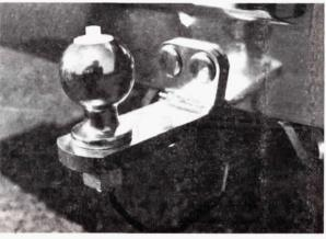
Here's a new trailer ball hitch that sounds your automobile horn if the hitch begins to come loose on the road, or if someone tries to steal the trailer while its hooked to your car.
