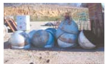
Schley cuts fire rings from 12 to 18 in. high (left). On other tanks he cuts off one end to make boilers, or both ends to make culverts.
