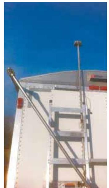
Each video camera is attached to a telescoping metal conduit that extends 2 to 3 ft. above the top of Jim Case's semi truck grain trailer.
