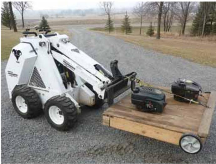
Dave Kulzer built this 40-in. wide, skid loader-mounted brush cutter out of wood. Loader forks slide through a pair of slots cut into back of deck.
