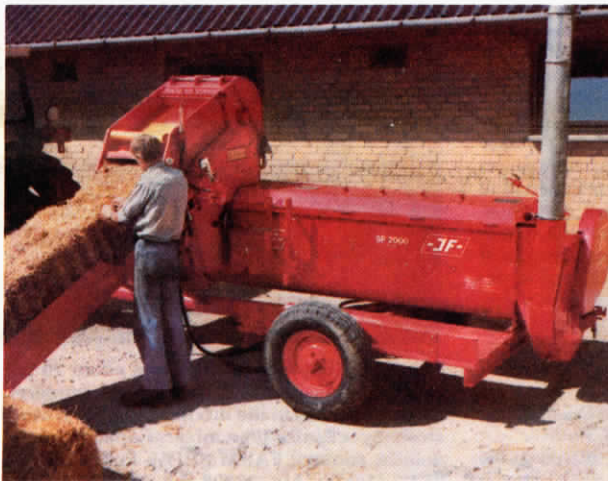
Capacity of this first-to-be-introduced straw processor is 2 to 2½ tons per hour.
