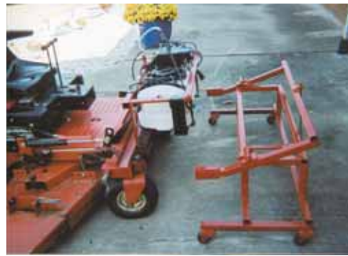
A 10-gal. tank and pump mount on a wheeled metal frame that attaches to zero-turn riding mower. A spray nozzle is located just outside mower's left front caster wheel.
