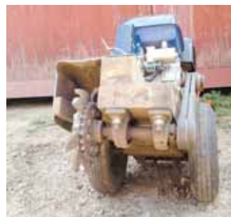
Stump grinder is powered by a 13 hp engine, which belt-drives the grinder's teeth.
