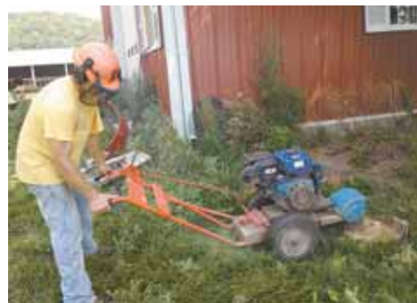
Tim Gasser built this walk-behind stump grinder that rides on wheelbarrow tires and uses the handles off an old rototiller.
