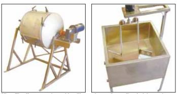
Kleen-Flo offers processing and handling equipment for small-scale dairy producers, including this 25-gal. butter churn (left) and square cheese vat.
