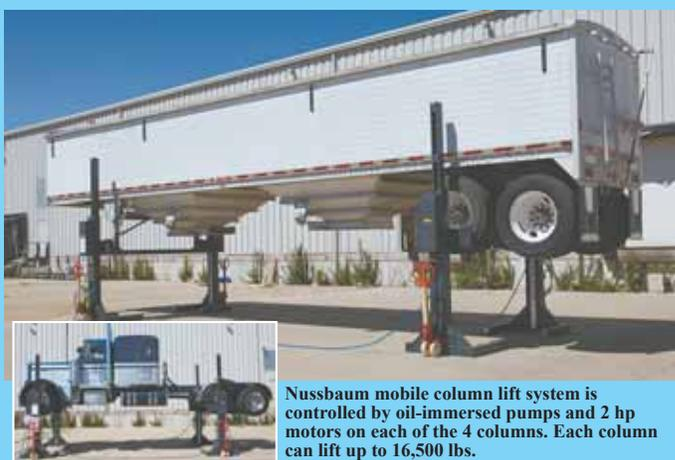
Nussbaum mobile column lift system is controlled by oil-immersed pumps and 2 hp motors on each of the 4 columns. Each column can lift up to 16,500 lbs.
