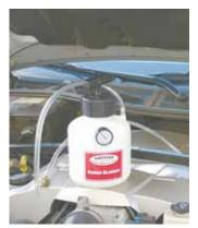
Power Bleeder consists of a pressurizer jug with a hand pump and pressure gauge, bleeder tubes, and a hose with a cap fitting to match the brake cylinder reservoir neck.
