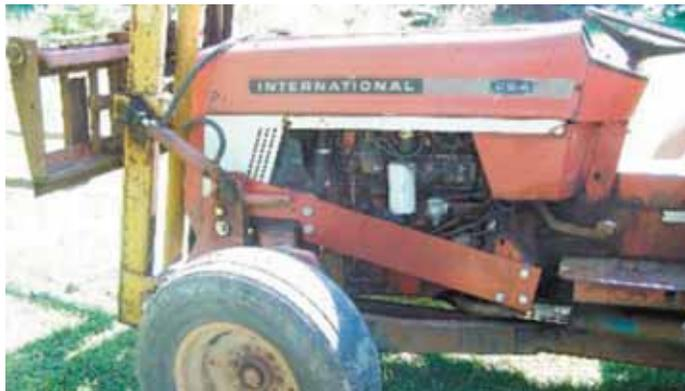
When the bolster on front of his IH tractor broke due to an overloaded forklift, Arthur Kidder made a heavy-duty repair that's strong enough to carry nearly any load.
