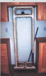
builder and needed to set kitchen cabinets in place without having to hire someone. So, I used built this 'cabinet jack' using pvc tubing and plywood. It mounts on 4 rollers. The legs are made from 4 lengths of 2-in.
