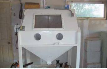
James Osnes used weldable industrial plastic instead of steel to build this big sandblasting cabinet. "The plastic has held up well with no chipping," he says.
