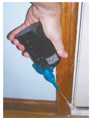
Smoke Pencil works great to find leaks that let in cold air in the winter and hot air in the summer.
