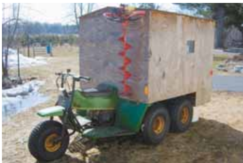
Gator-mounted, self-propelled ice fishing shack is made from treated plywood. A large ice auger stores on brackets mounted on front of shack.
