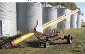
Brent Litke made this auger mover out of an old riding mower. "I stand next to the auger and use toggle switches inside a control box to control all operations," he says.
