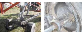
He stripped mower down to the front wheels and axle, then built an A-frame that attaches to auger frame. A belt-driven shaft runs through the transmission to drive both wheels.
